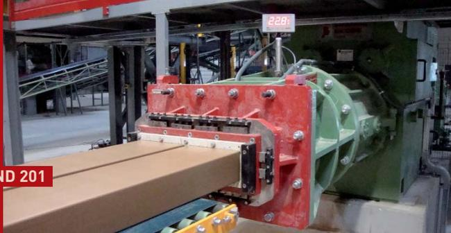
This patented system grants The constant feeding of the quantity of clay to the extrusion die, that means:
